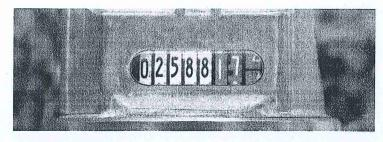
Water meters record the amount of water each premises uses. The black digits in the white area indicate kilolitres used (1,000 litres) and the white digits in the red area indicate litres used.
