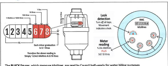
The **BLACK** figures, which measure kilolitres, are read by Council half-yearly for water billing purposes. The **RED** figures represent fractions of a kilolitre which may more easily indicate a water leak.
