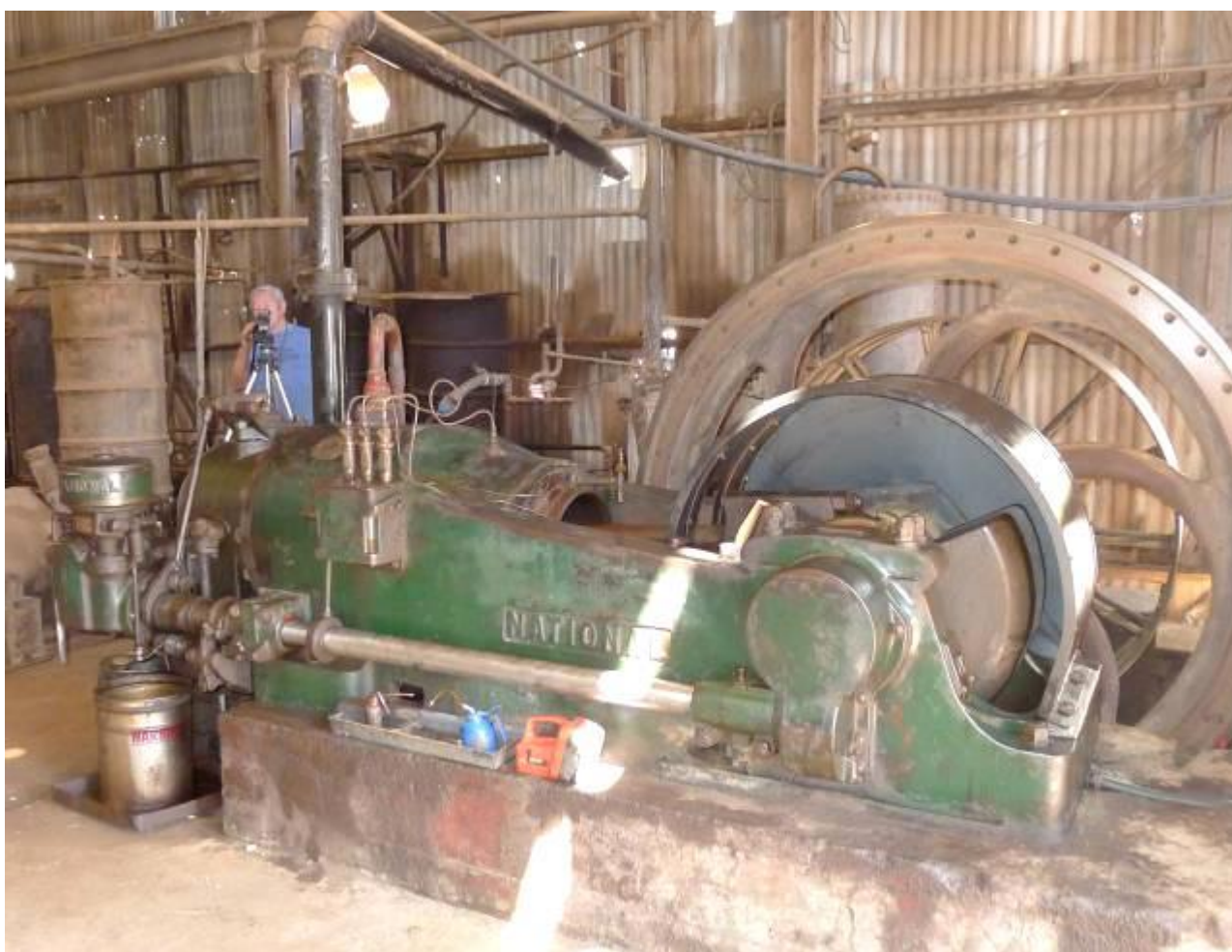
Figure 18: Comet Gold Mine National Diesel Power Engine
