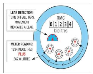
The BLACK figures, which measure kilolitres, are read by Council half-yearly for water billing purposes. The RED figures represent fractions of a kilolitre which may more easily indicate a water leak.
